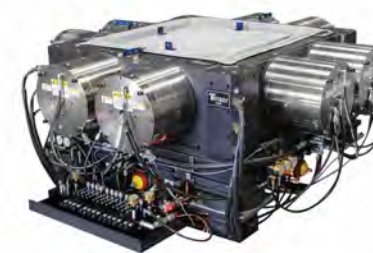
Sandia used a six-degree-of-freedom high-frequency vibration shaker to test the mechanical response of a nuclear deterrence modernization unit.
