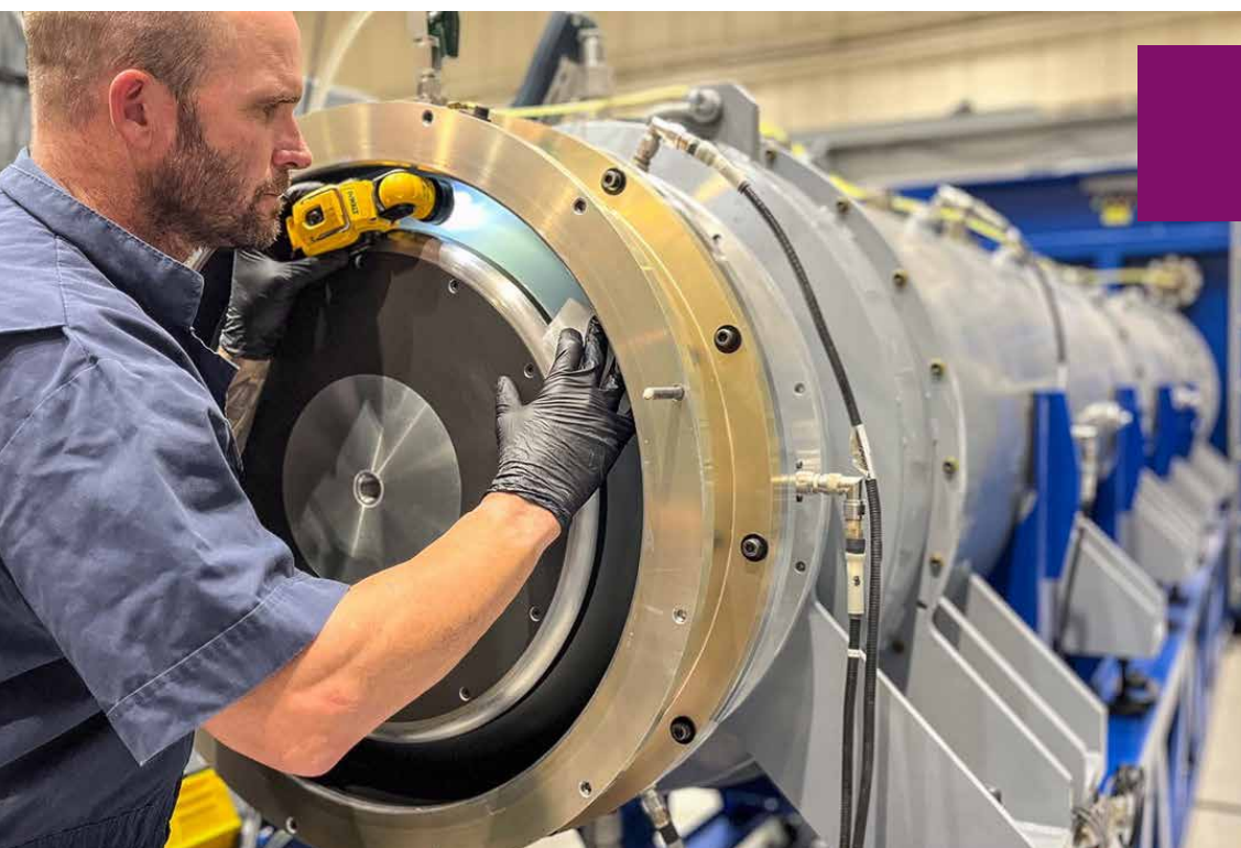
A technologist inspects the vacuum insulator on the front of Vulcan for damage and signs of electrical breakdown after a 1.5 megavolt test.
