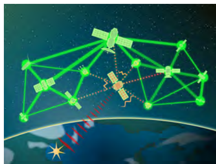
A cluster of relatively small and inexpensive satellites share data to work together as a single, autonomous unit.
