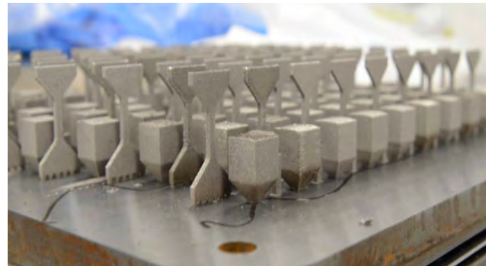
High-throughput tensile bar testing of Kovar samples is one component of multimodal data used to develop machine-learning models and process optimization within Hierarchical MultiLayer Algorithms.
