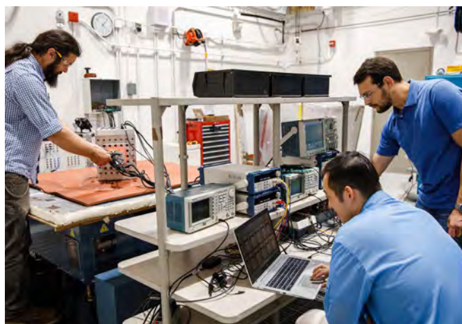
Staff members conduct shock and vibration qualification testing on the last development build of the W80-4 joint test assembly telemetry.
