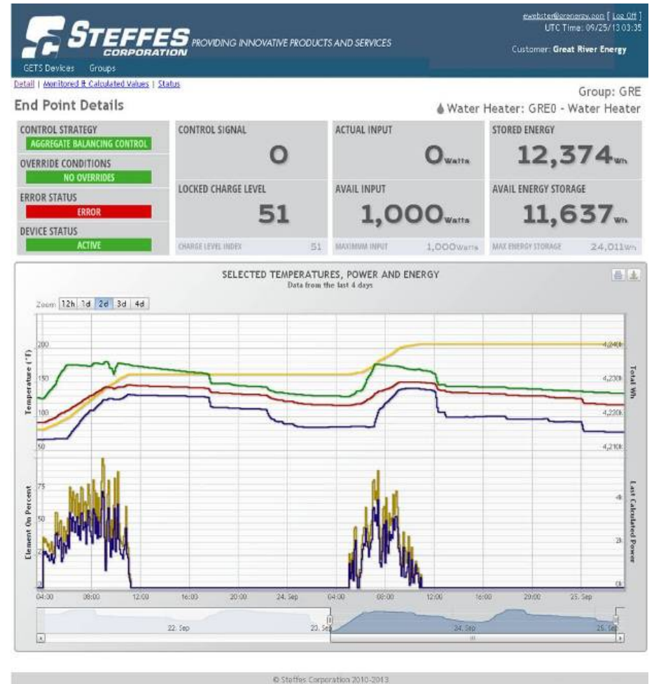
Steffes Data on Temperature, Power, and Energy for an Individual Water Heater
