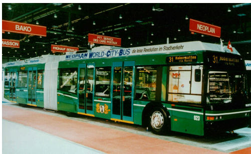
Figure 4: Basel trolley bus equipped with Magnetodynamic Storage system MDS K3
