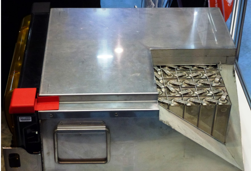
Figure 3. An FZSoNick 48TL200 sodium–nickel battery with welding-sealed cells and heat insulation. 2012 Image by: Rudolf Simon–Own work, CC BY-SA 3.0. ( https://commons.wikimedia.org/w/index.php?curid=18740786 )
