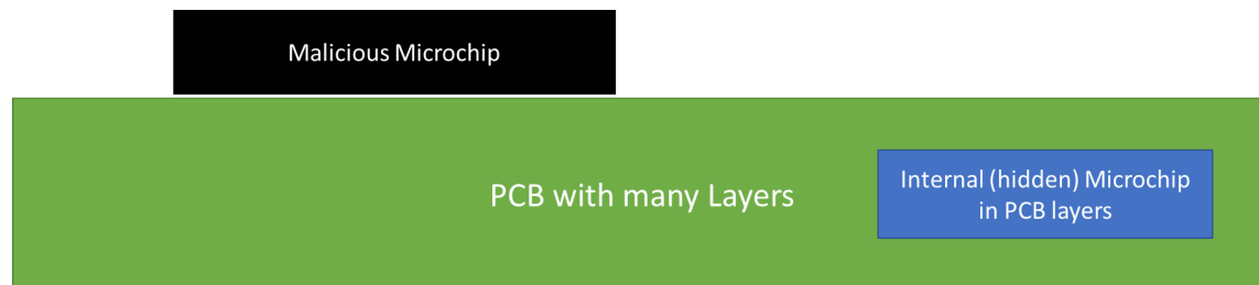
Figure 5-1. Layered Printed Circuit Board (PCB) with added malicious microchips
