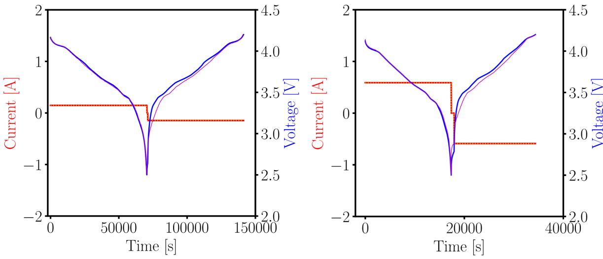
The experimental data for discharge at C/20 until 2.5V followed by 600 seconds rest and charge at C/20 until 4.2 V was used for optimizing the physics-based simulation parameters. Then the parameters were tested for a C/5 discharge-rest-charge cycle. Results show an RMSE of 1.4 % and an R<sup>2</sup> metric score of 0.98.
