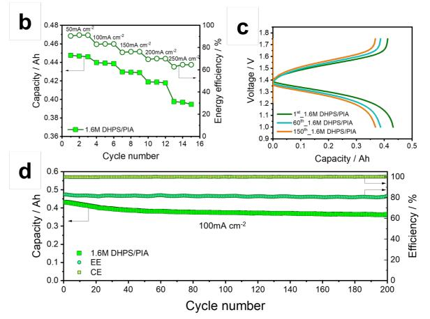
Stable cycling stability and good rate capability with high capacities at all current densities (only about 12% of capacity decay from 50mA cm<sup>-2</sup> to 250 mA cm<sup>-2</sup> current densities)
