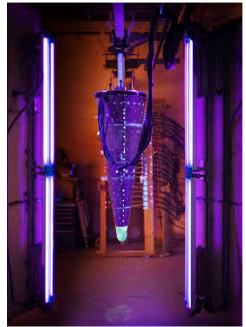
BLACK LIGHT EXPOSURE — During an impulse test at the Light Initiated High Explosives facility, a test unit is sprayed with a sensitive explosive and exposed to ultraviolet lights to enhance energy absorption. Photo by Craig Fritz
