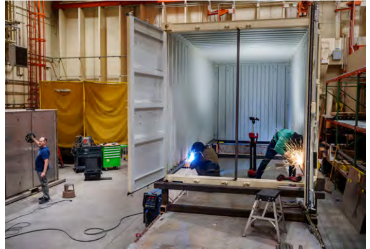
BUILD OUT — Two technologists weld the Mobile Vault frame to the exterior Conex container. Outside the container, an engineer performs a 3D scan of the Mobile Vault.
