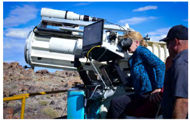
A CLEAR VISION — Laura McGill gets firsthand operator experience with Jim Rini in a ME-16 telescope during a visit to Tonopah Test Range in May 2022. The telescope is used to provide high speed documentary video. Photo by David Coleman
