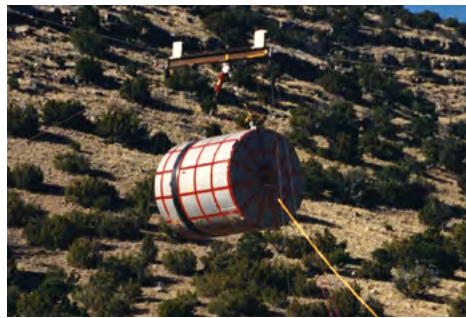
A TEST OF ENDURANCE — A TRUPACT-II container conditioned to minus 20 degrees Fahrenheit drops 30 feet onto a steel puncture bar multiple times at Sandia’s Coyote Canyon test facility in 1989. Photo by Randy Montoya
