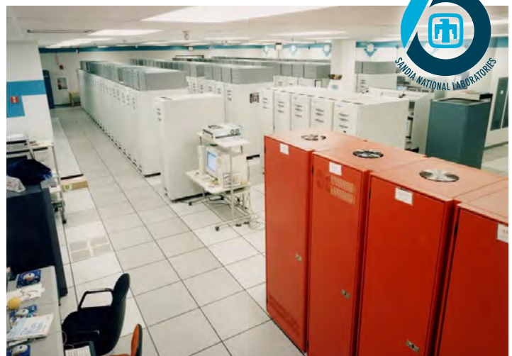
ASCI RED — Pictured in a photo from 2000, Red was a massively parallel computing system deployed by Sandia and Intel Corp. in 1996 to support the Accelerated Simulation and Computing Initiative program. It was the first computer to reach 1 teraflops computation and the first system in ASCI.
