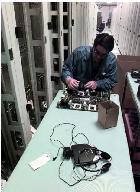
THE MOTHERBOARD — In a 1999 photo, a technician installs a processor on the Accelerated Simulation and Computing Initiative Red motherboard. Photo from the Lab News archives
