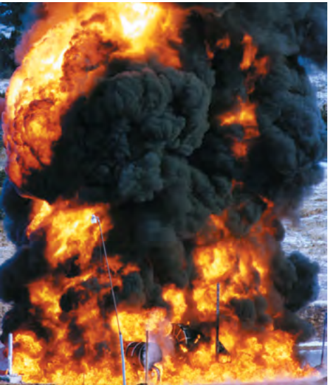
TESTING THROUGH FIRE — A TRUPACT-II container undergoes a fire-test with the goal of surviving 1,475 degrees Fahrenheit for at least 30 minutes without losing vacuum.
