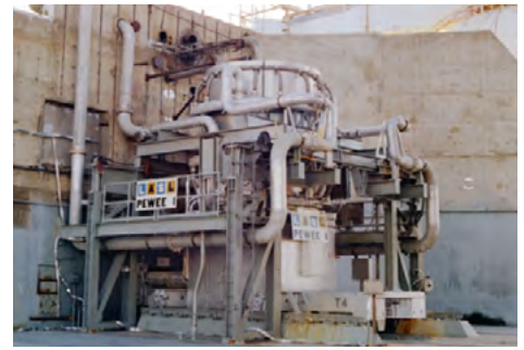
POWER TO SPARE — Testing of the nuclear rocket prototypes reached its zenith in 1968 with Phoebus-2A, roughly four times more powerful than a modern nuclear reactor but far more compact. Its successor, Peewee, achieved temperatures of 4,500 degrees Fahrenheit and tests showed its potential for space travel.
