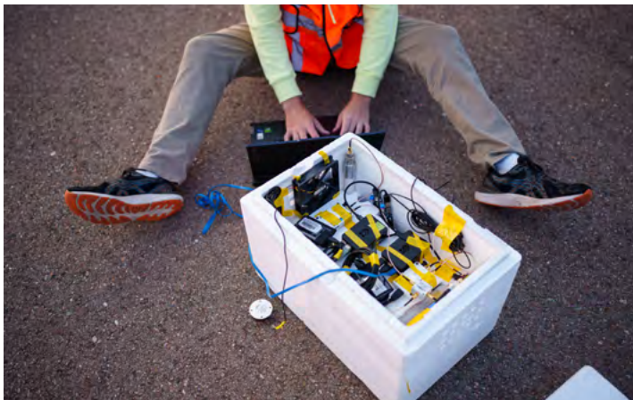
PACKING — Sandia intern Will Barrett prepares the payload for launch. The payload records GPS and non-GPS signals. After the flight, researchers compare their calculations from non-GPS signals to the actual positions.
