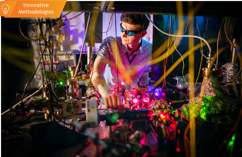
LASER SHOW — Dan Thrasher looks to his computer monitor while setting up an optical table at Sandia, where he is testing lasers in combination with barium ions to reduce drift in miniature atomic clocks, making them more accurate. Photo by Craig Fritz
