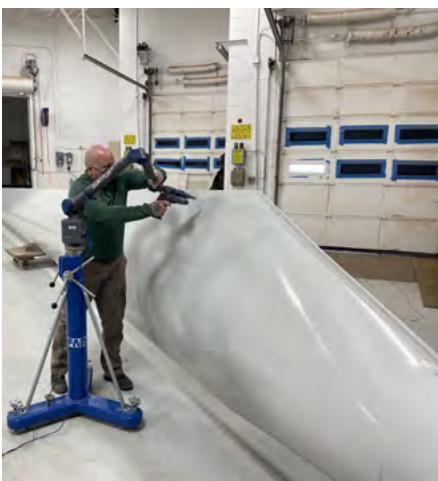
WELL SUITED — Point cloud scans were made before and after cutting away the outer shells of the blades to allow new 3D printed tips (left) to be perfectly mated to the blade root (right). In the future, researchers hope to use the blade root to test different tips.
