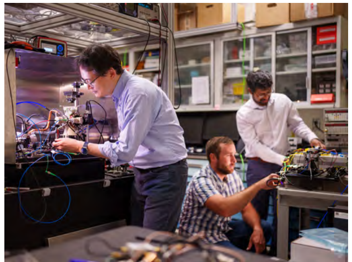
PREPARING THE EXPERIMENT — Sandia scientist Jongmin Lee, left, prepares a rubidium cold-atom cell for an atom interferometry experiment while scientists Ashok Kodigala, right, and Michael Gehl initialize the controls for a packaged single-sideband modulator chip. Photo by Craig Fritz
