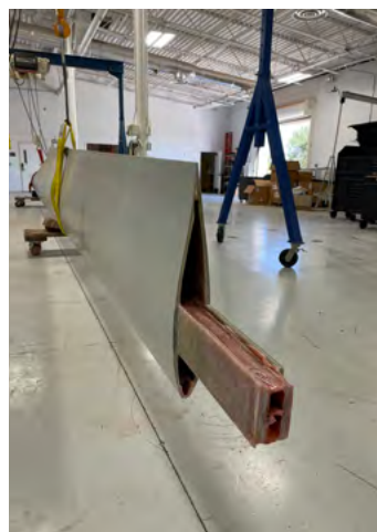
WELL SUITED — Point cloud scans were made before and after cutting away the outer shells of the blades to allow new 3D printed tips (left) to be perfectly mated to the blade root (right). In the future, researchers hope to use the blade root to test different tips.
