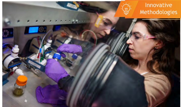
BETTER BATTERIES — Sandia battery expert Melissa Meyerson works in a glovebox to set up a lithium-sulfur flow battery. These kind of batteries have huge potential for being large, safe and inexpensive backups for a high-renewables grid. Photo by Craig Fritz
