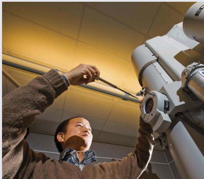
THREADING THE NEEDLE — Jianyu Huang demonstrates insertion of a sample holder into a transmission electron microscope at CINT. (Photo by Randy Montoya)
