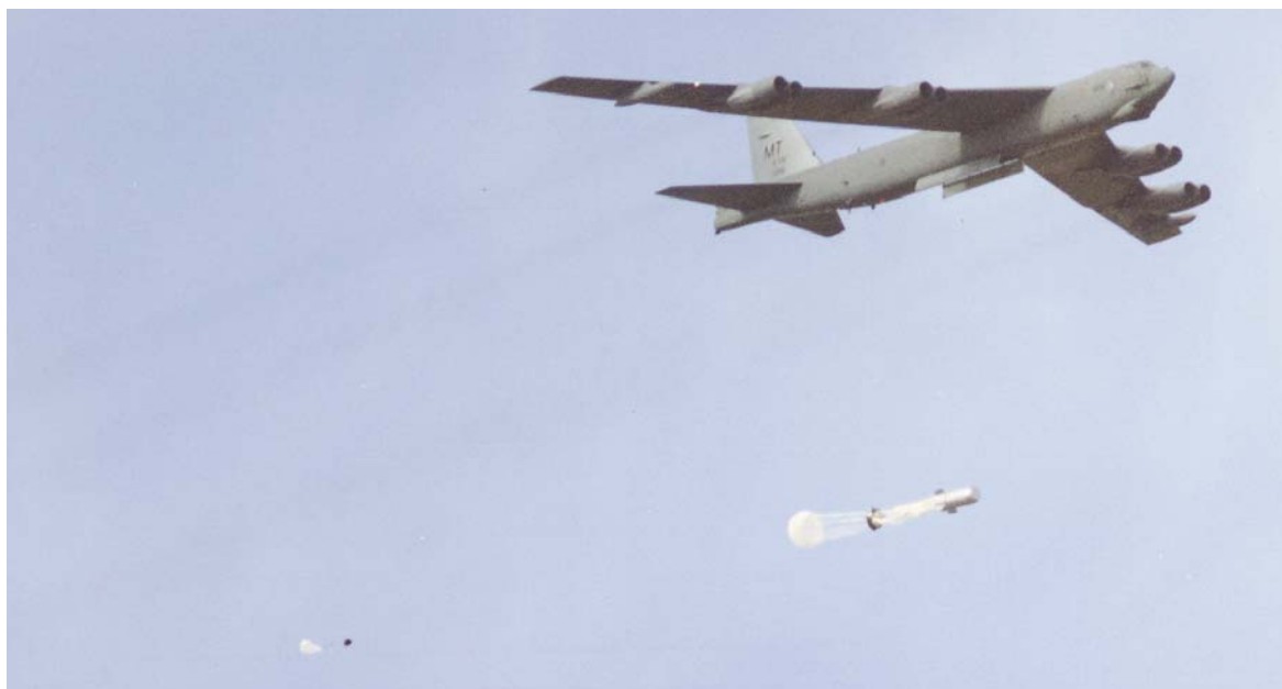
A B-52 CONDUCTS A DROP TEST of the B53 at the Tonopah Test Site during a 1995 test series. Note at lower left the drag chute, which deploys first and pulls the main parachute from the weapon casing.
