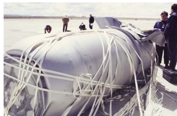
A MISSION TEAM inspects a B53 weapon casing after a test drop at the Tonopah Test Range in April 1995.
