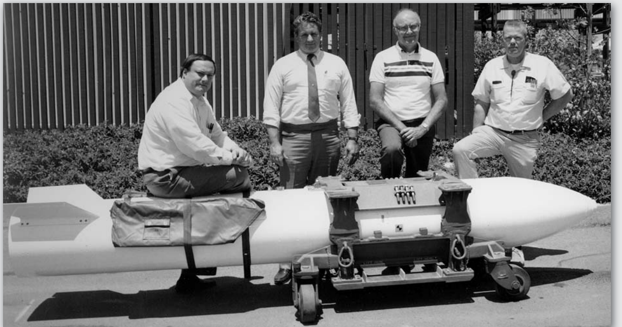
The B83 was the first megaton-class bomb to be specifically designed for laydown against hard, irregular targets. From left to right: Don Starkey, Jim Wright, Kurt Franklin, and Jerry Hunting with the B83 in 1980.
