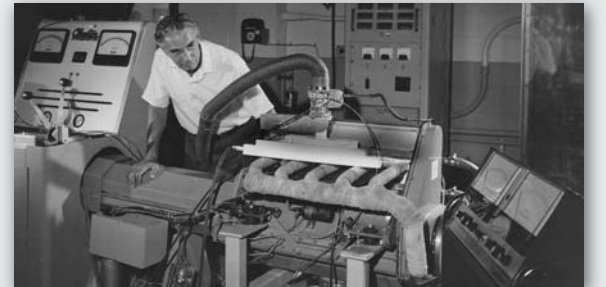
Inventor Harvey Pouliot and the variable displacement engine. In 1976, Sandia designed, built, and tested the engine that, according to computer projections, would have averaged 40 percent better gas mileage than a conventional engine of equal performance.
