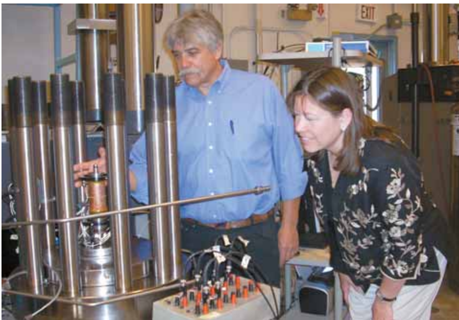
STEVE BAUER AND GEORGIANNE PEEK look at equipment that will be used to analyze core samples from the potential Iowa aquifer compressed air energy storage site. The data will provide necessary fundamental information used for the design and performance of the underground air storage vessel. (Photo by Chris Burroughs)
