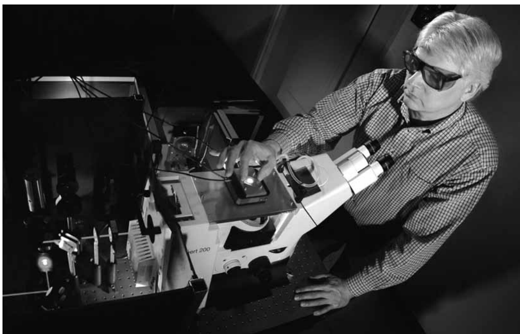
RESEARCHER CARL HAYDEN (8353) positions a lipid nanotube sample on the spectrally and lifetime-resolved confocal imaging microscope. (Photo by Randy Wong)
