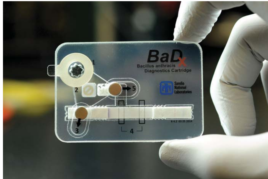
SANDIA'S BaDx pocket-sized detector has everything needed to test a sample for anthrax.
