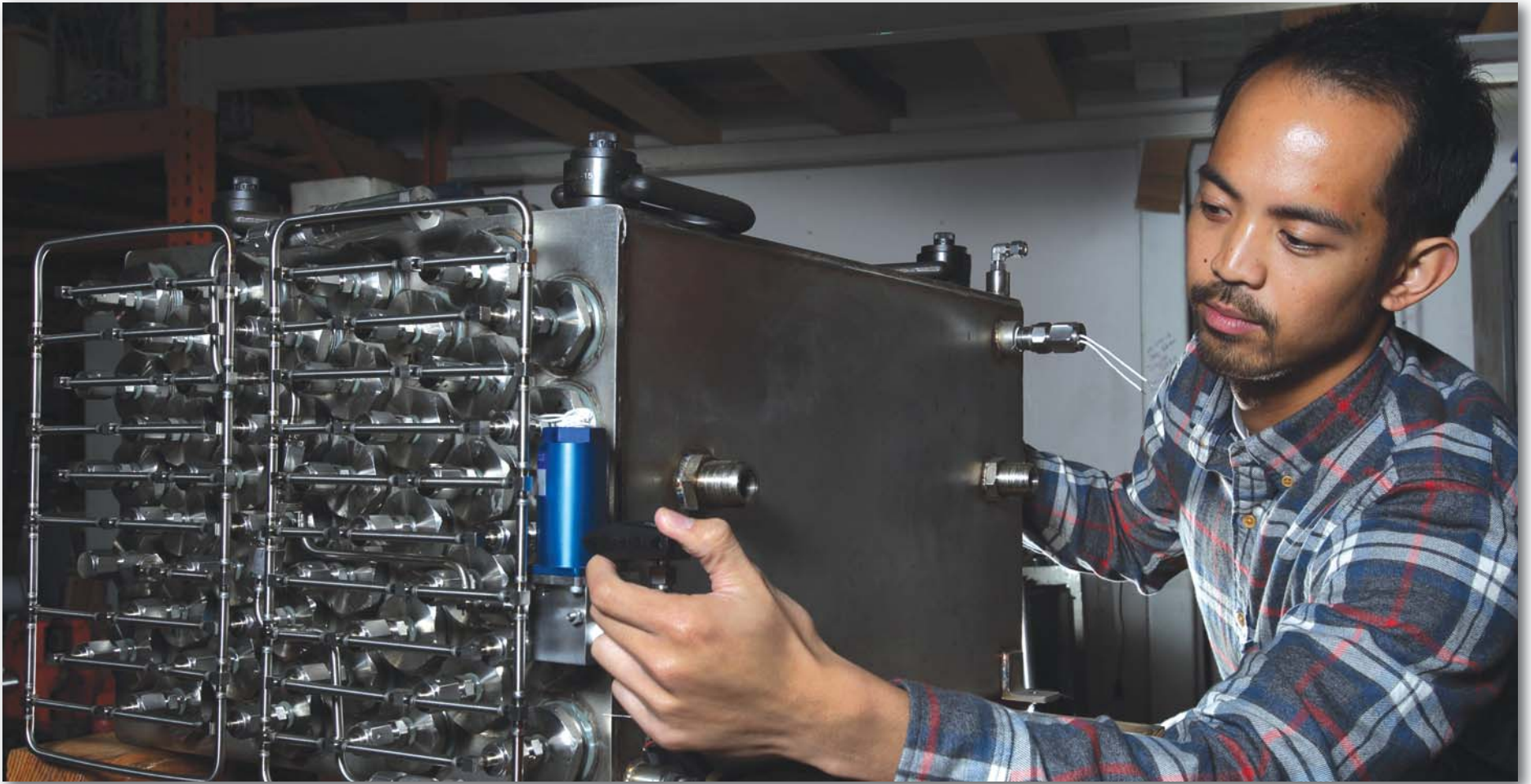
ADRIAN NARVAEZ of Hawaii Hydrogen Carriers (HHC) observes a metal hydride storage tank, part of a project led by Sandia. The tank will be combined with a fuel cell system to make a fuel cell power pack to power a forklift. Hydrogen fuel cell technology could have a significant advantage over batteries for a large slice of the $33 billion US forklift market. (Photo by Dino Vournas)
