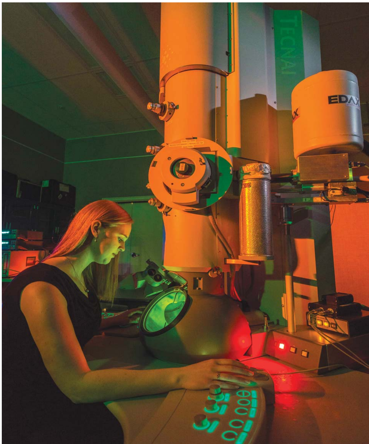
SANDIA'S KATIE JUNGJOHANN (1132) sends electrons through materials to analyze their structure at the Sandia/Los Alamos-run Center for Integrated Nanotechnology. (Photo by Randy Montoya)
