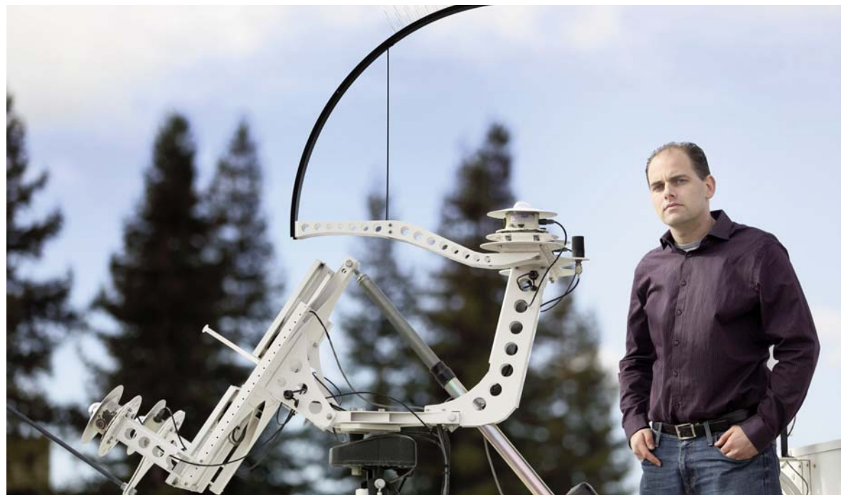
MATT LAVE (6112) uses pyranometers like these to measure the amount of irradiance, or available sunlight. There are four round pyranometers, capped by small glass domes, on this device. The work by Matt and Josh Stein (6112) shows that the variability of a point sensor is larger than the variability of a PV power plant. (Photo by Dino Vournas)
