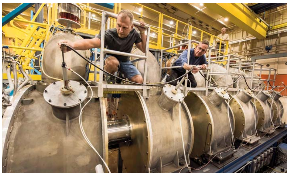
RITS-6 AT WORK — Derek Ziska, left, and Dan Nielsen (both 1656) stand on the pulse-forming line platform to check the magnetic core reset mechanism on the RITS-6 cavities as Advanced Radiographic Technologies manager Mark Kiefer (also 1656) looks on from the walkway above. RITS-6, a flash X-ray source, has operated for about a decade and recently fired its 2,000th shot.
