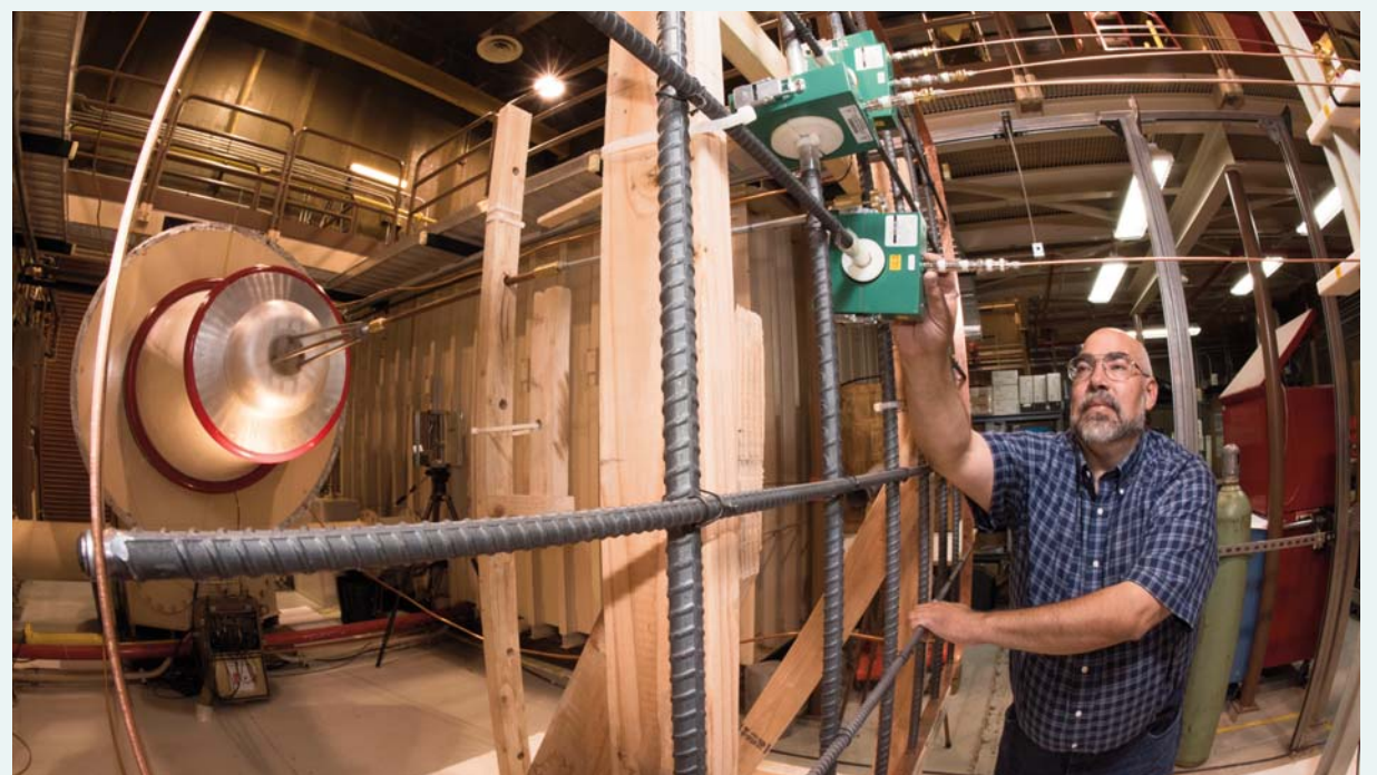
RESEARCHER LEONARD MARTINEZ makes an adjustment at the Lightning Simulator lab as part of a test series to further knowledge of lightning protection systems by looking at how lightning currents flow through rebar lattice structures. Sandia's specialized lightning lab evaluates how everything from sensitive nuclear weapons components to entire buildings will hold up against the worst that nature can offer. (Photo by Randy Montoya)
