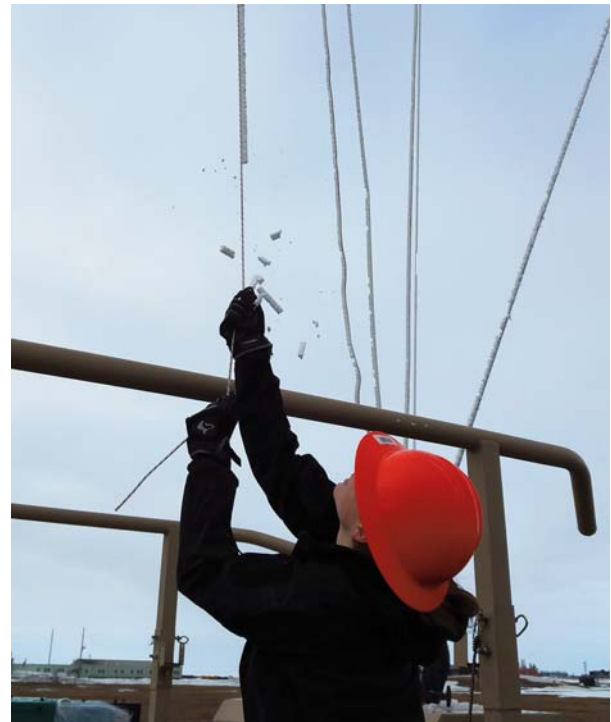
A CASCADE OF ICE breaks loose from tether lines as Darielle Dexheimer gathers in an instrumented balloon at the ARM research station at Oliktok Point, Alaska. The balloon is about 25 feet above Darielle's head and the lines are completely iced over. (Photo courtesy of Darielle Dexheimer)
