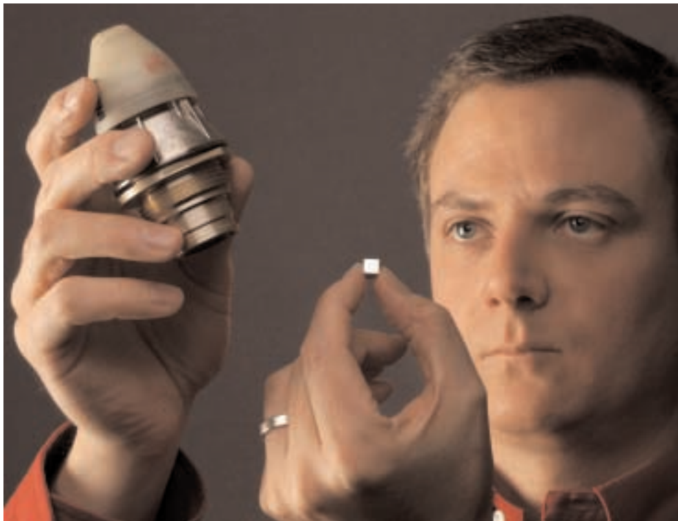
SAFE, ARM, FUZE AND FIRE – Darren Hoke (2614) holds the before and after of this important military weapon component. The quarter-inch cube represents the new real estate Sandia designers are targeting using microelectromechanical systems (MEMS) technologies.
