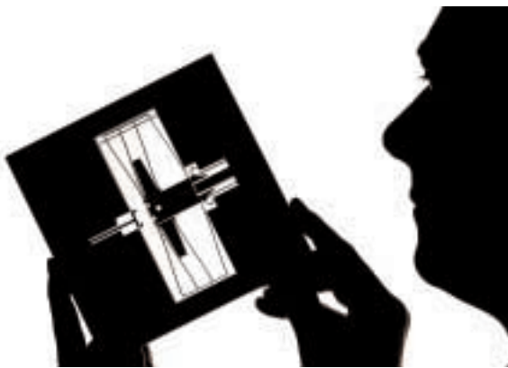
MACROVIEW OF MICROFUZE— The actual three-layer MicroFuze device designed and fabricated at Sandia is considerably smaller than this macro-model, examined by Darren Hoke (2614). The microsystem approach to sensing acceleration and spin may have other weapons applications in addition to the fuzing system.
