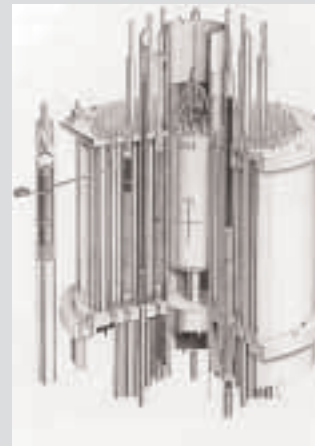
ACRR CUTAWAY: The illustration shows a cutaway view of the ACRR. Visible are the fuel rods extending above the upper grid plate which supports the fuel elements. In the center is a central cavity that is where researchers typically put their experiments. To the left is an enlarged fuel rod with an enlarged fuel pellet.
