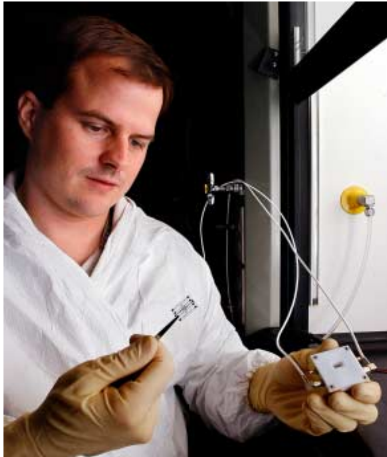
DARREN BRANCH conducts an experiment with the lipid bilayer biosensor that has the promise of rapidly detecting a variety of biological agents, including viruses, anthrax, and other bacteria. (Photo by Randy Montoya)
