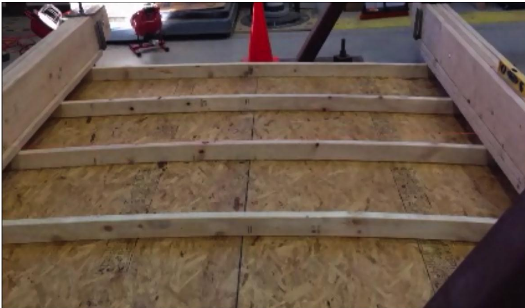
Figure 15. Photograph of roof assembly under load.
