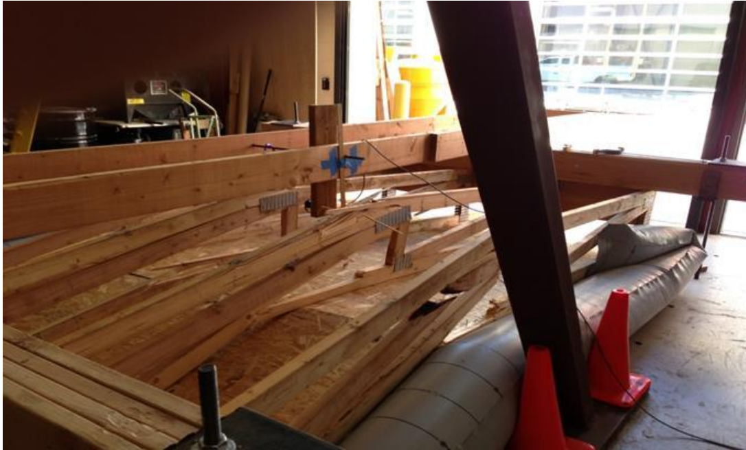
Figure 27. Failure in open web (web member) truss roof test assembly.
