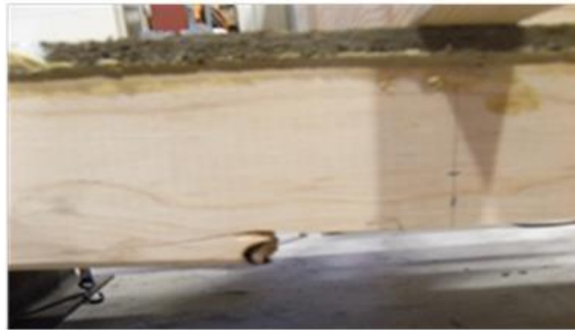
Figure 3. Sketch of cracks in tested joists, and photo of typical crack initiation at knot on tensile face of joist.
