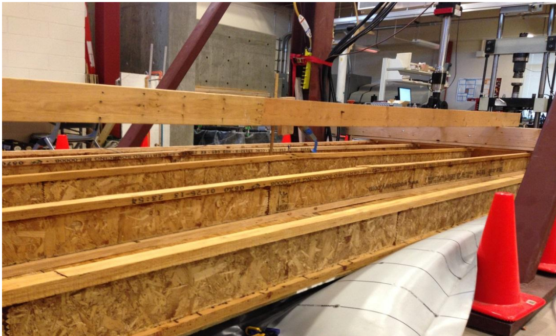
Figure 29. Failure in TJI roof test assembly.
