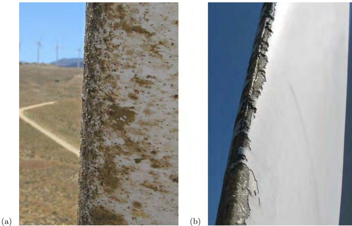
Figure 1.1. Wind turbine blade roughness. Roughness here is of (a) insect or (b) erosion type [44, 35].
