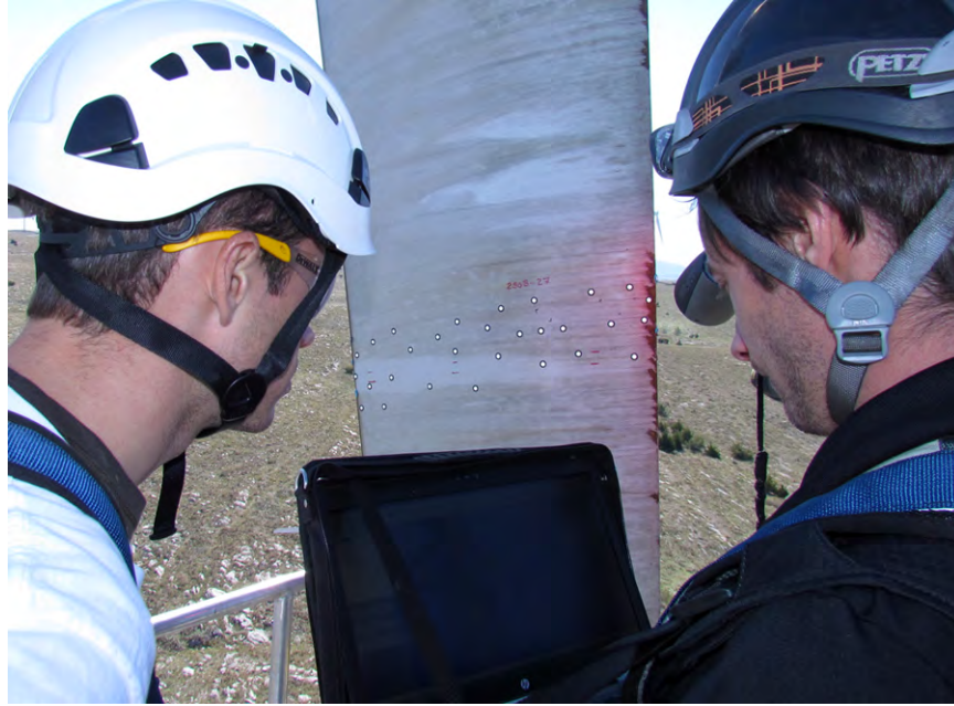
Figure 2.7. Example the ExaScan measuring erosion on a blade segment.
