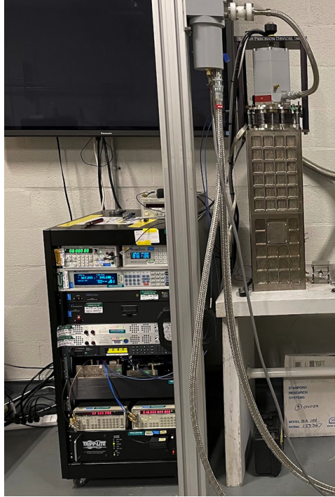
Figure 4: Complementary measurements were done on a single TRISO particle in a relatively low-background laboratory at the ORNL Energy Systems Test Complex. The particle was packaged in a vial and placed on the table in front of the microcalorimeter and (not pictured) HPGe detectors.
