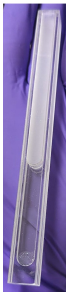
Figure 3-2. Photograph of optically transparent sapphire cell.
