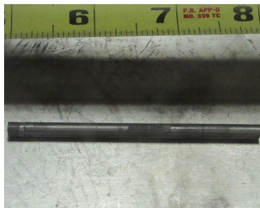
Figure 30. Depleted uranium-zirconium-molybdenum fuel rod used for salt processing studies in the MFIT
