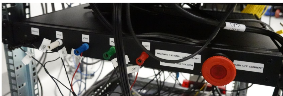
Figure 34. Argonne National Laboratory’s custom 12-channel multiplexer for controlling electrochemical sensors in the Kairos test loop.
