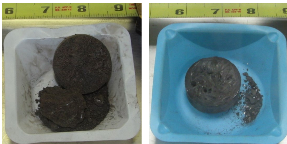
Figure 11. LiCl-KCl-UCl 3 (left) 72.3 wt% UCl 3 and (right) 60.8 wt% UCl 3 before and after electroanalytical experiments.
