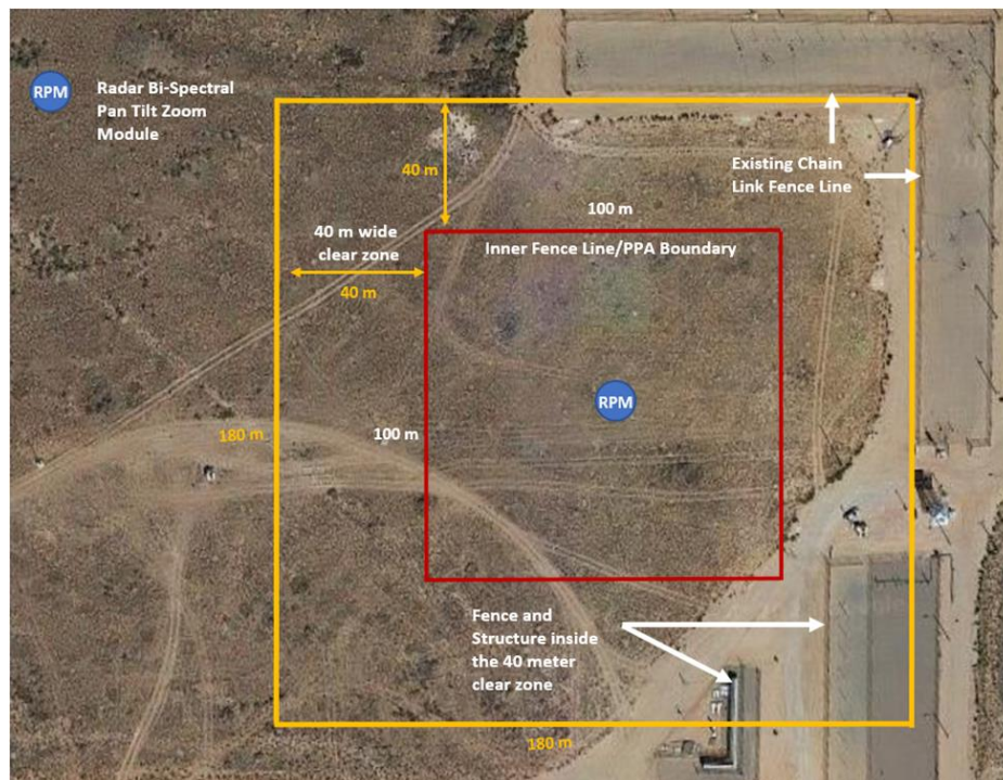
Figure 8: Test Bed Simulating an SMR Site Employing a DMA Design
