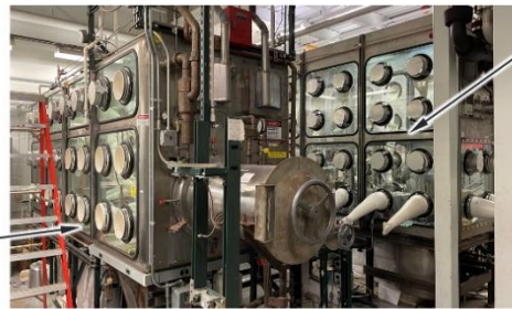
Figure 14: Modular Flow Instrumentation Testbed (MFIT) at Argonne National Laboratory. Rendering of the Platform (top), Storage Tanks and Associated Parts (Bottom Left), and Salt Purification and Flow System Glovebox (Bottom Right).
