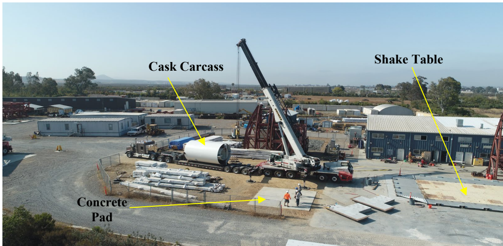
Figure 3-19. Cask arrival to LHPOST (UCSD).
