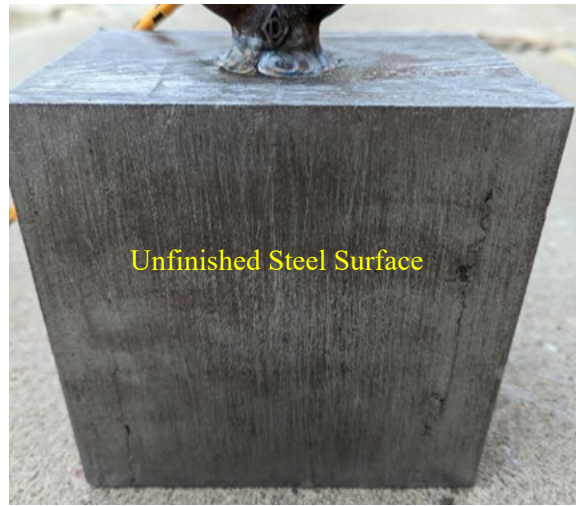
Figure 4-3. Steel block used in push-off friction tests.
