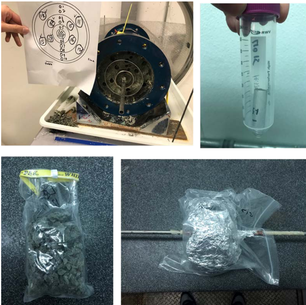
Figure 6-28. Images from dismantling of the HotBENT Lab #2 experiment. Clockwise from top left, (a) images of ring placement and map of sample removals, (b) sample removed for analysis, (c) residual central layer preserved for future analysis, and (d) bulk sample.
