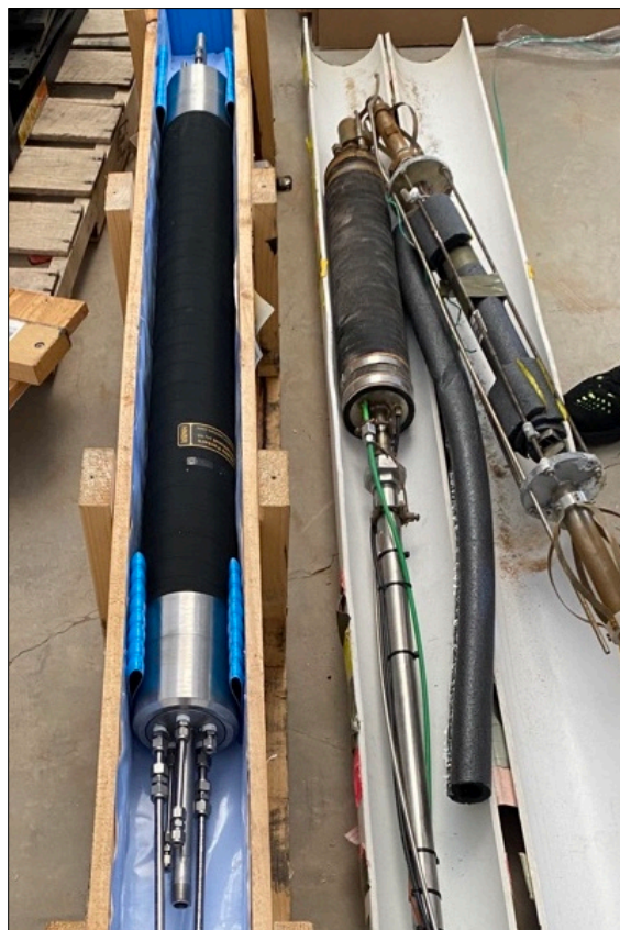
Figure 5. Comparison of BATS 1 Aardvark HP packer after removal (right, in pipe) with BATS 2 IPI packer before installation (left, in box).
