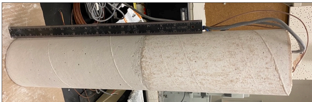
Figure 12. BATS 2 lab-constructed composite seal emplaced in SL borehole. Salt concrete (left) and sorel cement (right) were constructed in a single mold. Thermocouple (red) and strain gauge (gray) wires are visible coming out of the drift-side of the plug on the right. Ruler marked in inches.
