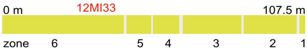
Figure 306. Position and dimensions of individual monitoring zones in borehole 12MI33.
