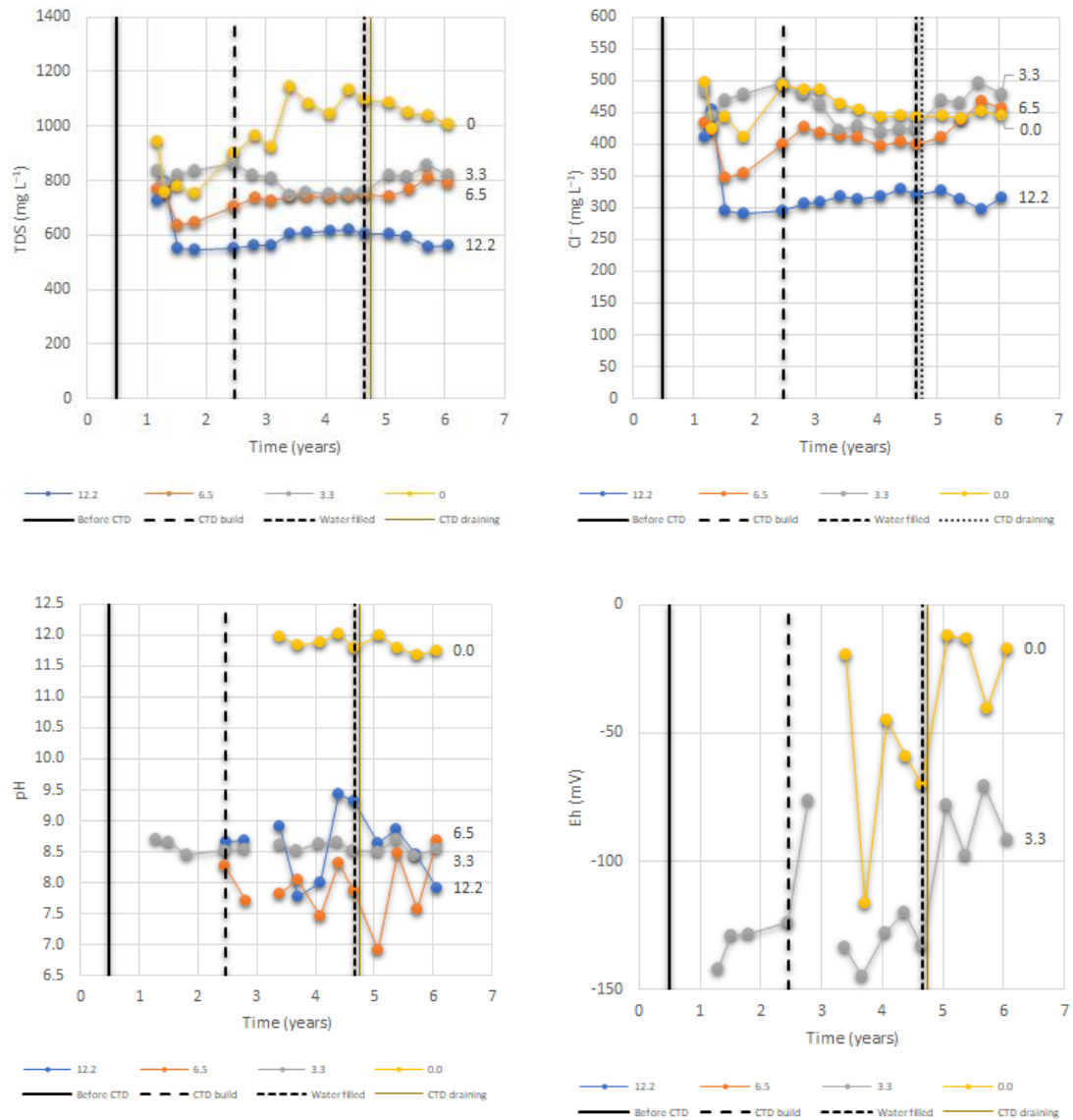
Figure 314. Time evolution of total dissolved species, Cl, pH and oxidation-reduction potentials in individual zones of 13MI39 borehole. The vertical lines indicate the stages of building a CTD.
