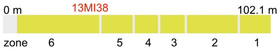
Figure 309. Position and dimensions of individual monitoring zones in borehole 13MI38.
