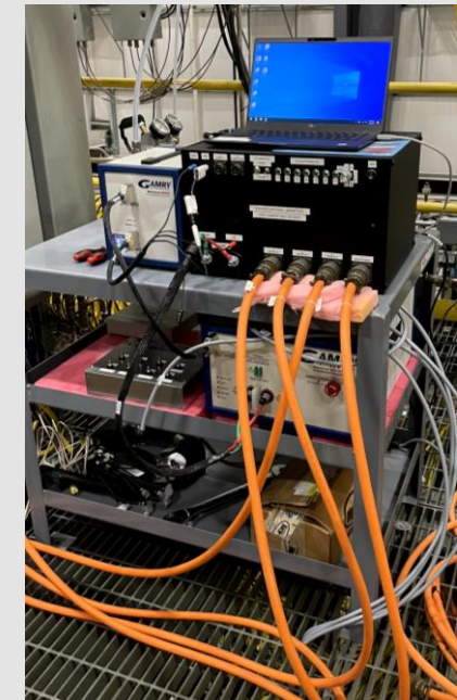
Kairos Power's Engineering Test Unit 1 and electrochemical sensor instrumentation
