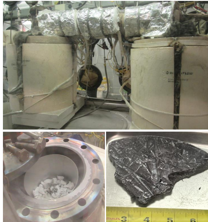
MFIT for fuel-bearing salts (top), As-received MgCl_2 -KCl-NaCl (bottom left), MgCl_2 -KCl-NaCl with 2.0 wt% UCl_3 (bottom right).
