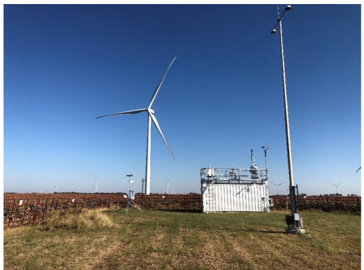
Image of AWAKEN Site A1, showing an instrumented turbine with nacelle mounted lidars and Atmospheric Radiation Measurement (ARM) mobile facility with scanning lidar and additional meteorological instruments. (Image by Thomas Herges)
