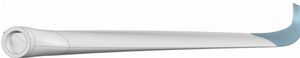
Rendering of the aeroshell of the AMSIT tip and winglet, mated to the base blade (Graphic by Brent Houchens)
