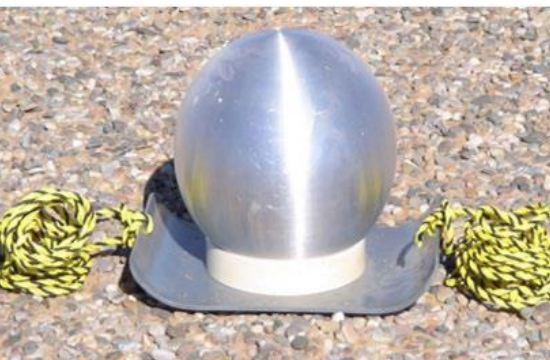
12-inch Al Ball to simulate belly crawl
