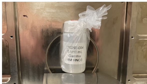
Figure 1: Dissolved AGR2 and AGR5/6/7 materials were packaged in plastic or glass vials for measurement.
