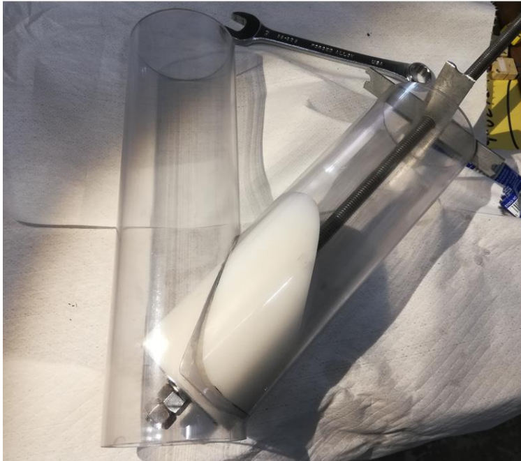
Figure 25. Assembly of Y tube using adhesive and alignment plug pull device
