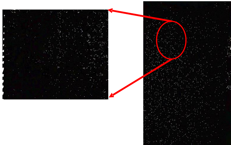
Figure 3. Images of a flat-surface graphitic surrogate impregnated with 2 mm diameter YSZ microspheres with an interstitial spacing of 3 mm.
