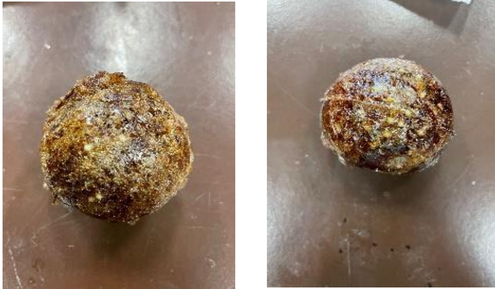
Figure 4. Completed spherical graphitic surrogates of pebbles embedded with 15 YSZ microspheres (left) and 30 YSZ microspheres (right).
