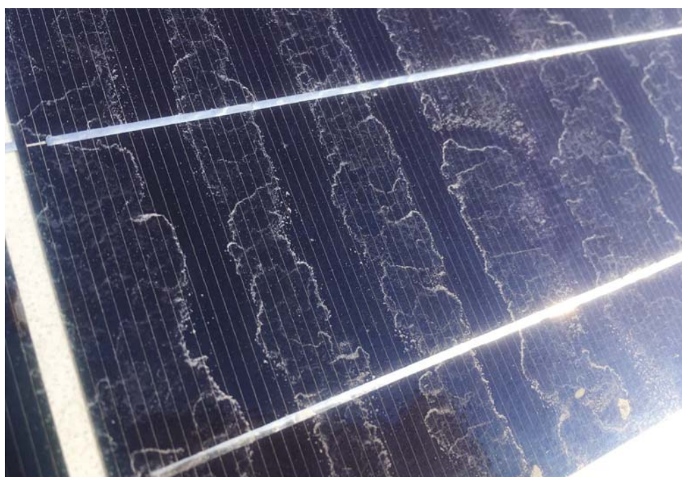
Figure 5. Condensation is important and complex in PV soiling because it can trap dust particles but also remove them
