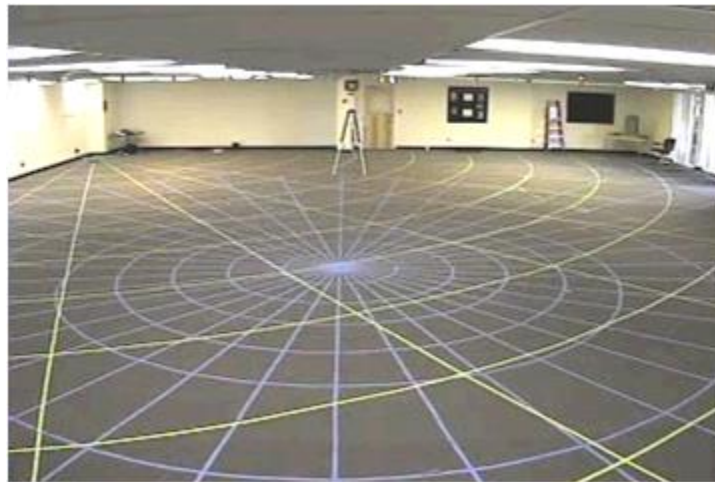
Figure 5-3. Example of a Test Grid Layout Using Tape
