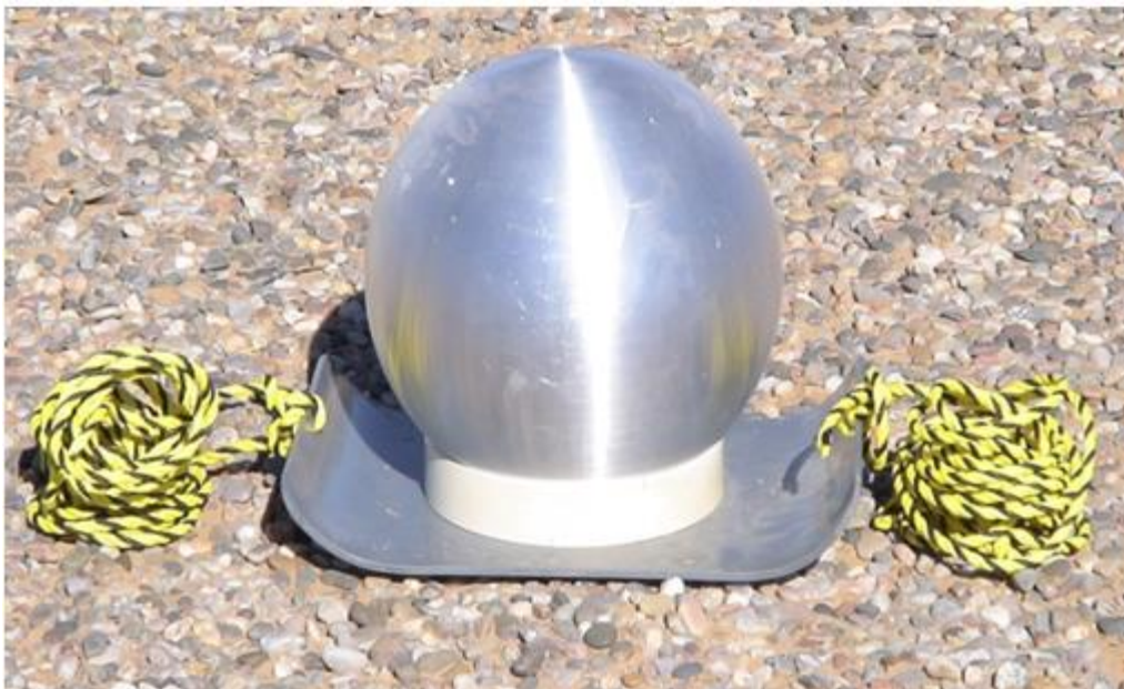
Figure 5-14. Aluminum Target Used for Microwave Testing
