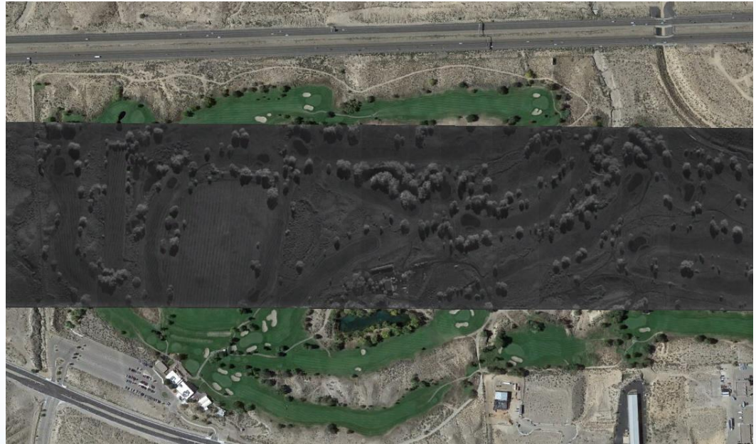
Ka-Band 4-inch resolution SAR interleaved stripmap, UNM Golf Course, overlay on Google-Earth.
