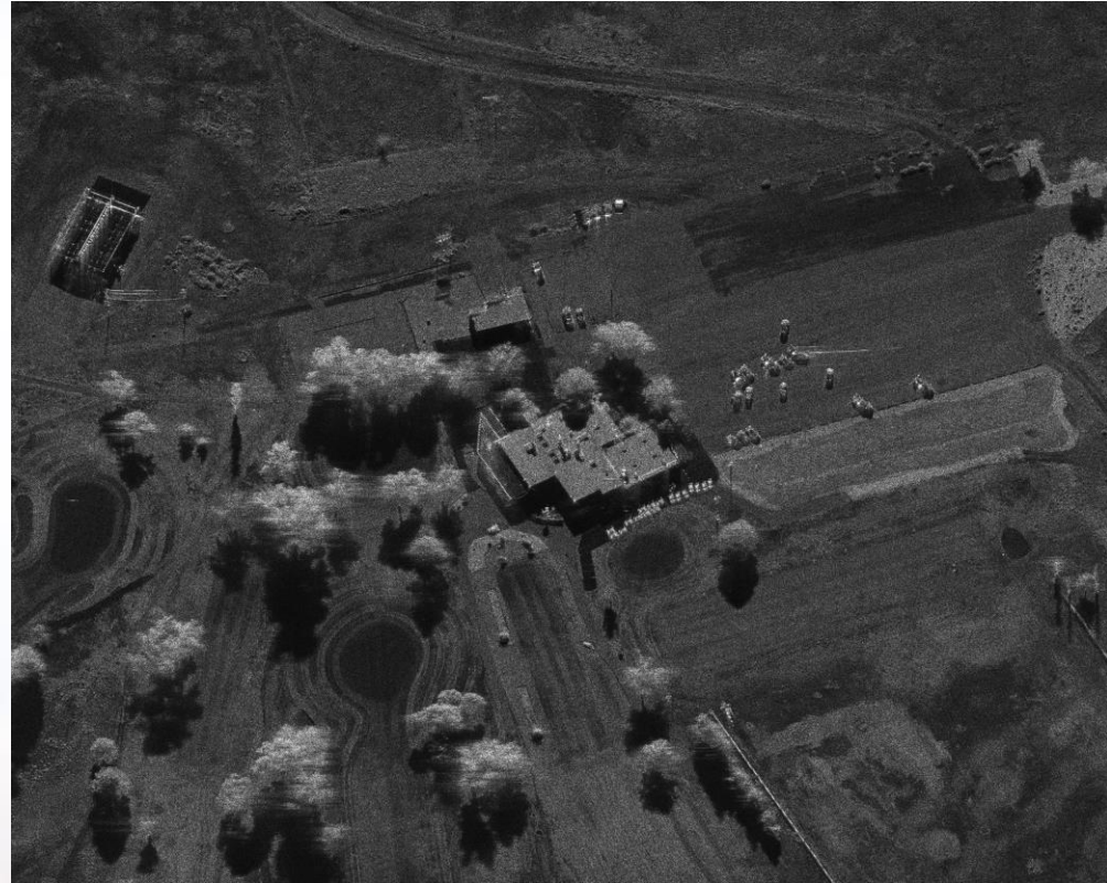
Ku-Band 4-inch resolution SAR image, Tijeras Arroyo Golf Course, KAFB, New Mexico
