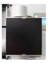
**The Gen 2.0 fixture** above integrates a full head form to integrate with commercial filtration testing – combining fit testing and filtration testing into a new, streamlined, and efficient approach.
