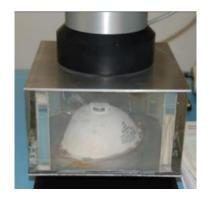
**Current N95 testing methods** shown above require a mask to be attached to a flat surface.
