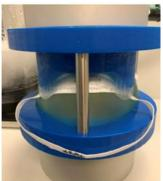
**The Gen 1.0 fixture** above tests masks performance on an enhanced mask form to emulate the human face. The testing device compresses the mask with 50 psi.
