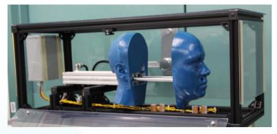
The mechanical test fixture shown above is designed to support the study of mask reuse testing, donning cycles, speed, and displacement.
