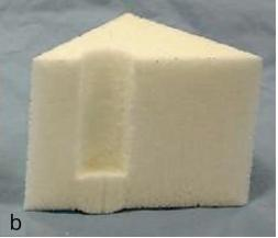
Samples of TufFoam<sup>™</sup> (a) and a TDI based foam (b) after being impacted with a plunger showing how TufFoam<sup>™</sup> is much more effective in spreading a penetrating load immediately after impact.
