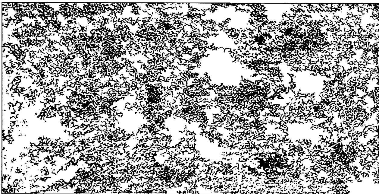
Figure 6. TCE distribution in the 15.4 \times 30.3 cm fracture prior to initiation of the dissolution experiment and simulation. Solid areas represent entrapped TCE, and open areas represent water flowing from left to right.
