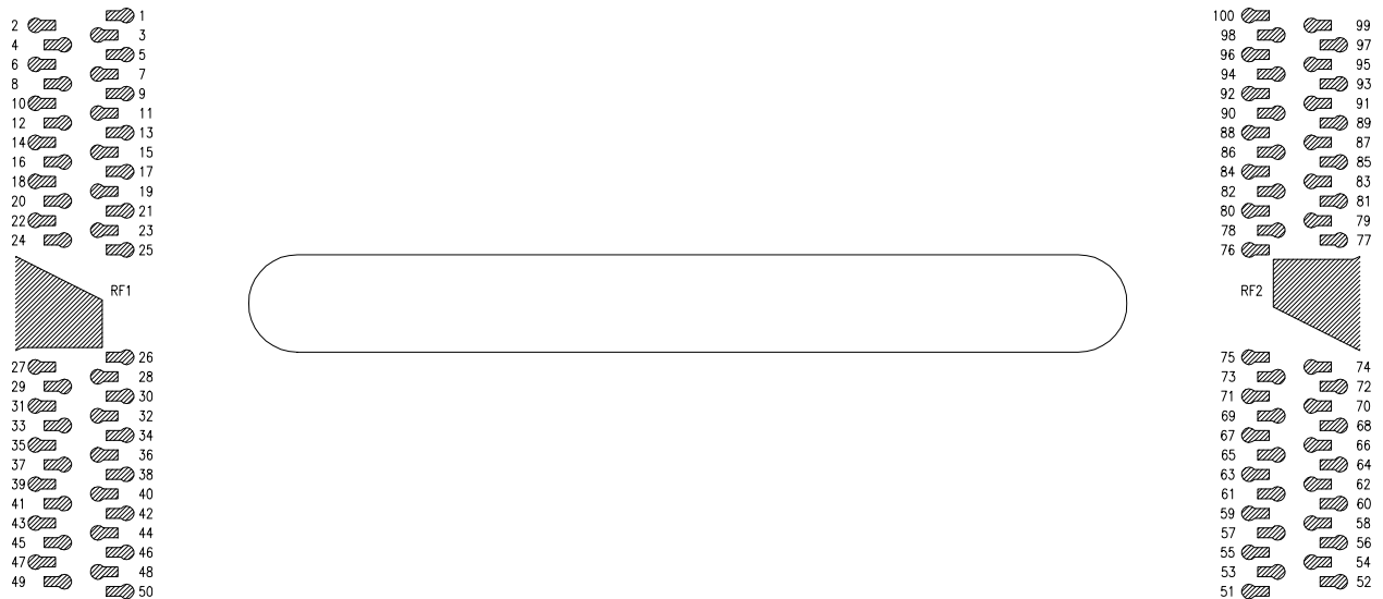
Figure 6-4.: Package Pads. Numbering of the pads of the Bowtie-102 package. The package provides 100 control signal bondpads, two rf bondpads (RF1 and RF2) as well as a ground plane (not shown here).
