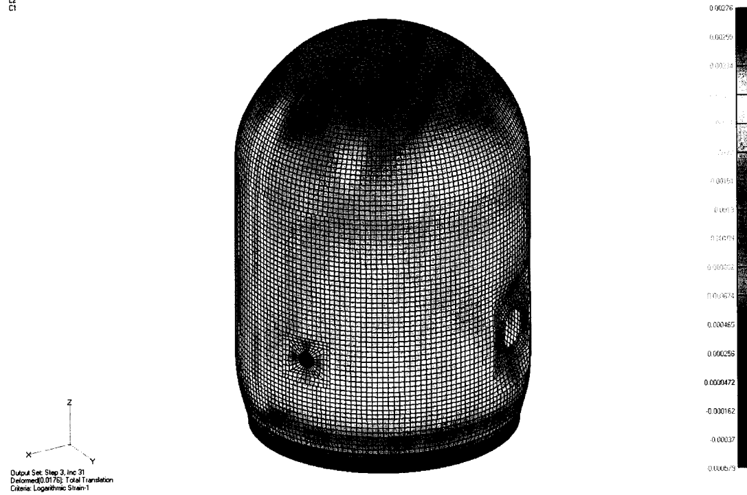
Figure 11 Case 1:Liner strain in circumferential direction at 1.0MPa – loading by pressure and temperature
