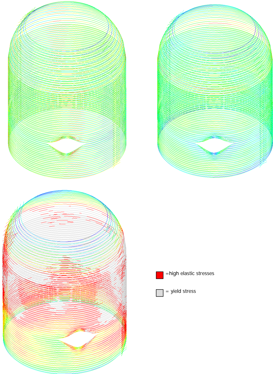
Figure 12.15 Stresses in tendons, case 2. Time = 0, 260.6 and 3600 minutes respectively.
