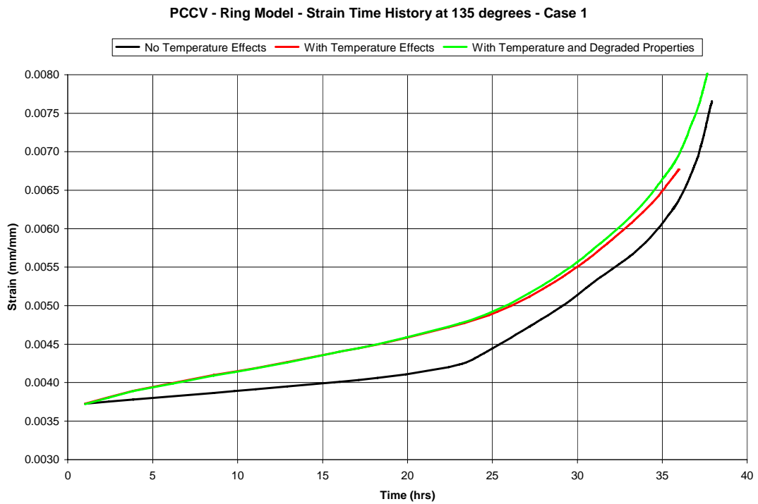
Figure 25. Hoop Tendon Strain History for Ring Model, Temp Case 1 Analysis, at 135-degree Azimuth
