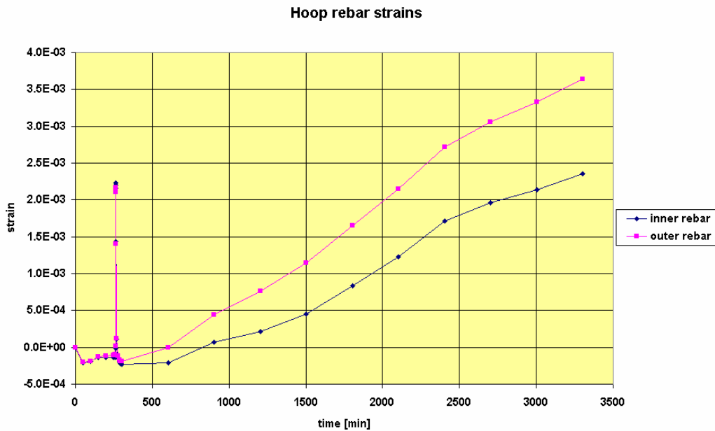
Fig. 58: Case 2, hoop rebar strains for inner and outer rebar, combined pressure and temperature loading (slice model) , position 6.2 m above top of basemat
