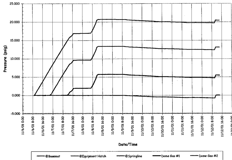
Figure 3.13 Pre-SFMT Hydrostatic Pressures
