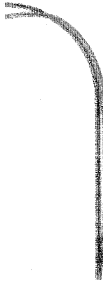
Fig. 6: Deformed model at 1.0 MPa (magnification of displacements = 50)
