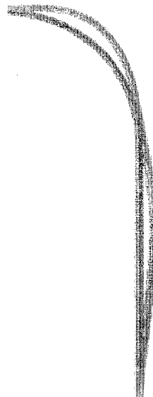
Fig. 8: Deformed model at 1.4 MPa (only in calculation, magnification of displacements = 10)
